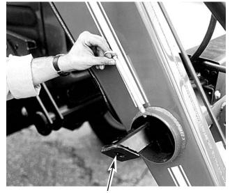
Fully Insert Stands And Pin Into Place
